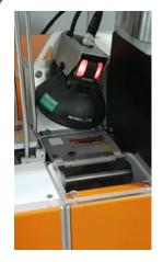
The vision inspection module includes a Keyence vision sensor that can manage OCR/OCV for readability of text, numbers, logos verification, bar code verification (1D, 2D like QR code), magnetic stripe detection, chip detection, etc.
